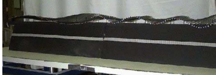
You can demonstrate: (1) wave propagation; (2) velocity in different media by two sections whose oscillators have different mass; (3) wavelength versus velocity and frequency; (4) reflection at fixed and free boundaries (by clamping the end if desired); (5) constructive and destructive interference; (6) standing waves and resonance (a mechanical oscillator for fixed known frequencies is available if desired); (7) reflection and transmission at media boundaries.
